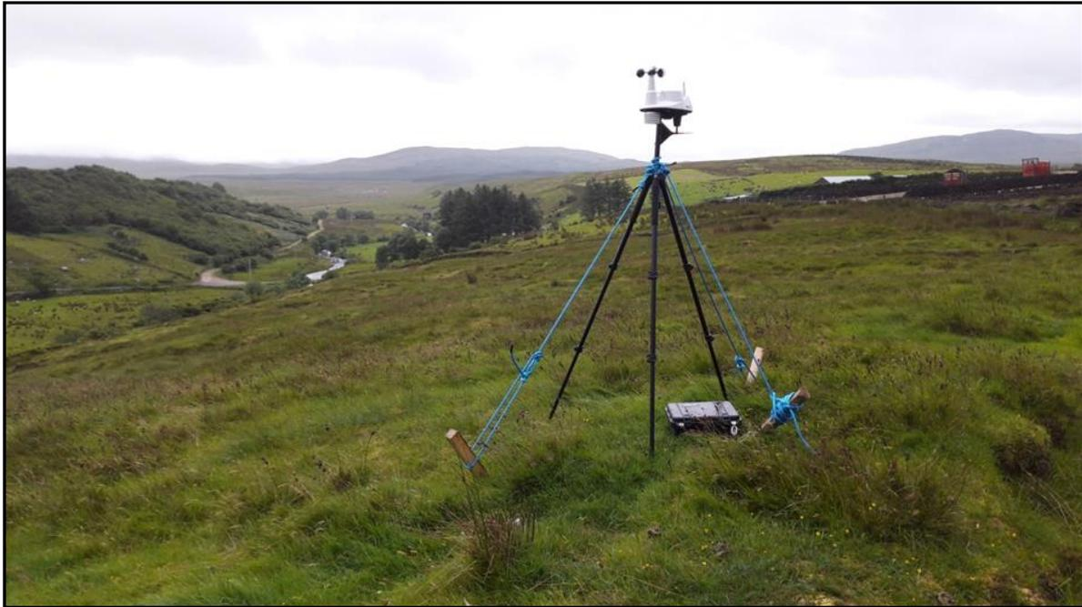
**Plate 5-4: Anemometer and Rain Gauge**
