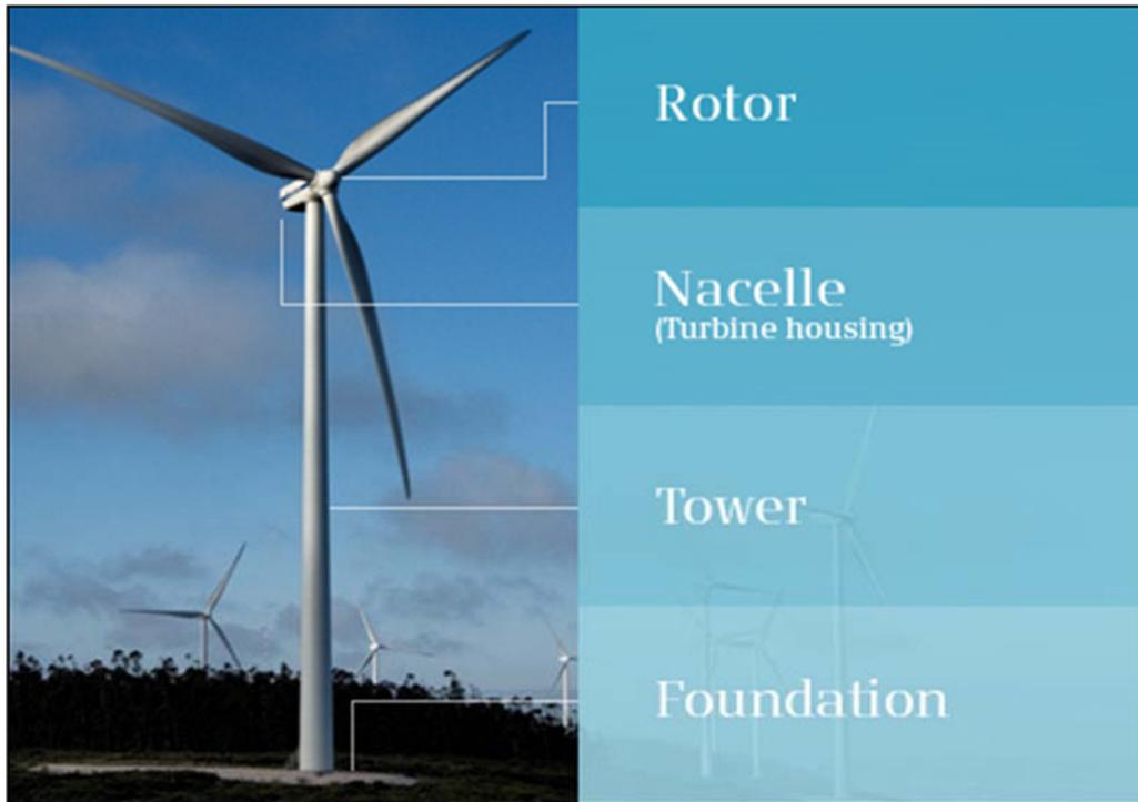
Plate 4-1 Wind turbine components
