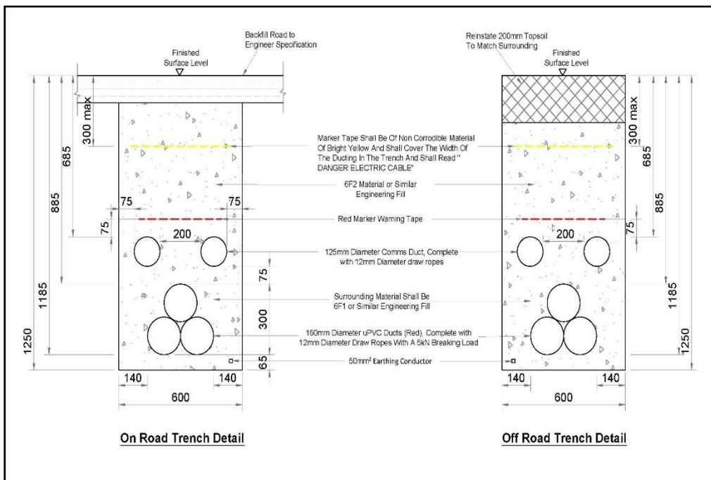
Figure 4-14 Typical Onsite Cable trench cross-section detail
