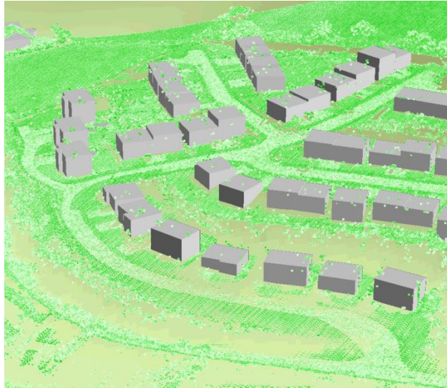
Figure 6-4: Sample Point Cloud from Aerial LiDAR Survey
