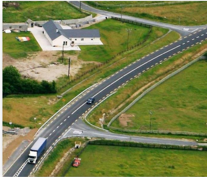
Figure 3-3: DN-GEO-03060; Simple T Junction with Right/Left Stagger
