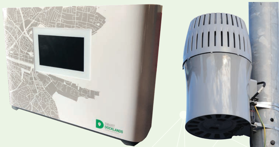
Examples of indoor (left) and outdoor (right) small cell solutions. Credit: Smart Docklands.
