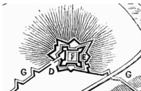
Fig.11: Henry Luttrell's 1689 plan of the town and forts of Sligo, as re-drawn by Wood-Martin, 1882-92, ii, p.134 depicts the fort with outer entrenchments with their own earthen bastions, and a fortified 'sally port' to allow troops in the Green Fort to reinforce troops in the outer defences.
