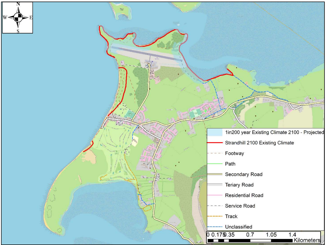
Figure 6.7: Summary of the coastal flooding risk at Strandhill with a 1 in 200 year existing climate flood event from tidal inundation shown
