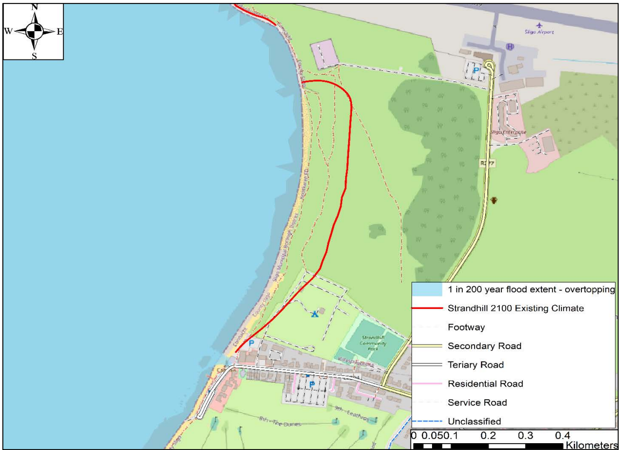
Figure 6.8: Summary of the coastal flooding risk at Strandhill with the 1 in 200 year existing climate flood event from overtopping shown
