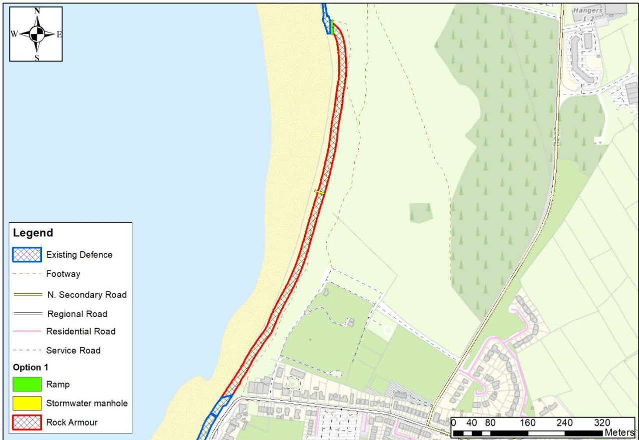
Figure 10.4: Location and extent of proposed CFERM option 1 at Strandhill town – a rock revetment solution
