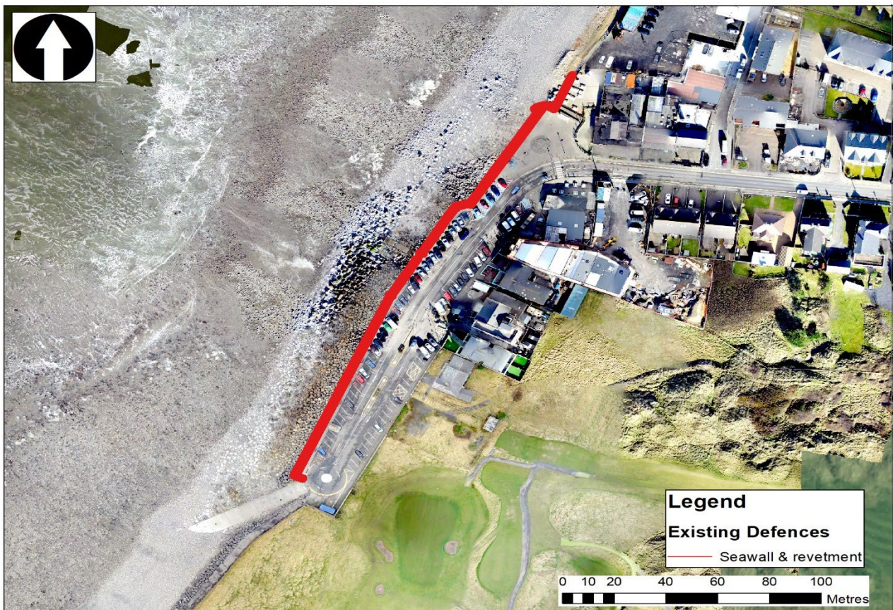
Figure 5.1: Location of the coastal defences at Strandhill whereby wave overtopping was assessed
